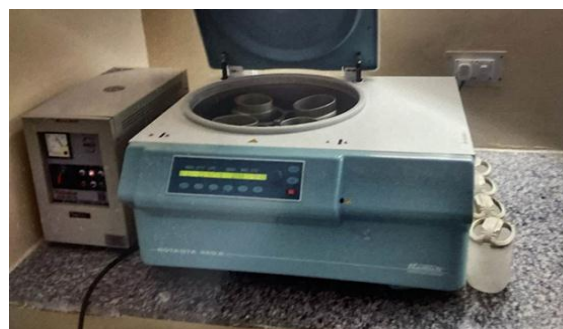
CENTRIFUGE (Rotanta 460 R, Germany) (with lid open showing centrifugation chambers)
